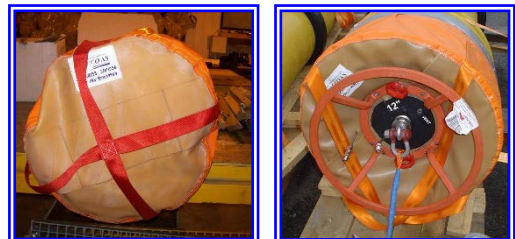
ROV Removable Ucaps for 12" Termination Heads with wire attachment (2 off versions)
