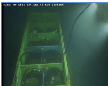
Basket with compartments for Electrical / Optical Flying Leads
