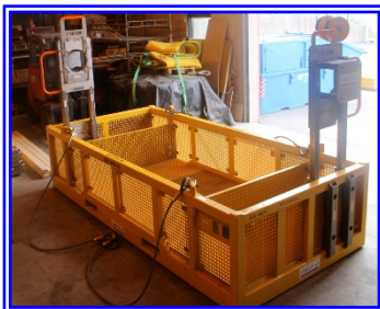
Ubas G with 2 compartments for combined EFL/OFL and HFL deployment / installation.
